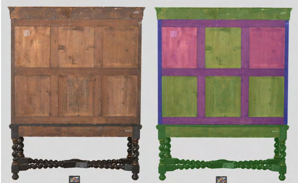
**Figure 3** The back of the cabinet. On the right, the different wood species of the framework are coloured in Photoshop CS5: green = softwood (presumably from the *Pinaceae* sp.), purple = beech (*Fagus* sp.), blue = oak (*Quercus* sp.) (note: the side panels are of softwood), orange = a light coloured hardwood, possibly poplar (*Populus* L.).
