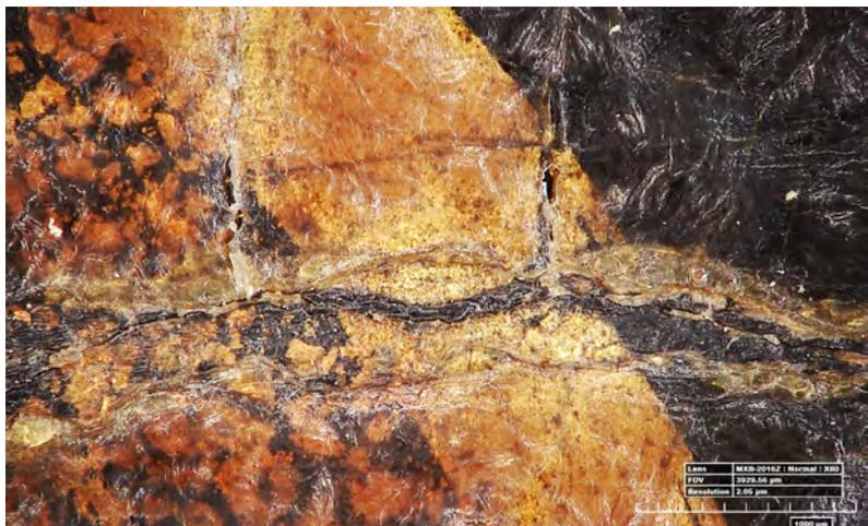
Figure 7 Detail of the metal particles (powder) and speckles of the 'gold' decoration on the right front door. A crack in the transparent lacquer layers runs horizontal through the picture, exposing the larger and irregular metal speckles to the left and the finer metal powder to the right. Hirox 3D-digital microscope, 80x, VIS.
